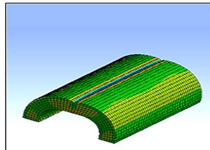
Figure 5. Maximum principal stress distribution for unstrengthened vault
