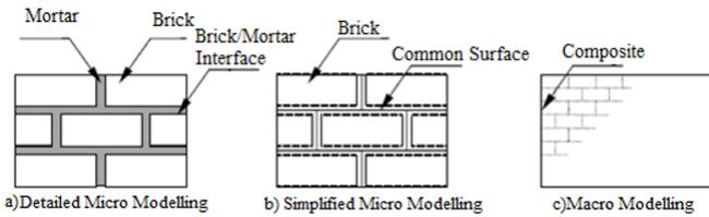
Figure 3. Modelling techniques used in masonry structures
