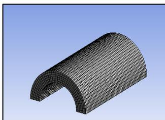
Figure 1. Vault model and mesh situation
