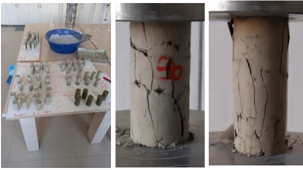
Fig. 3. Examples of studied samples and fracture patterns
