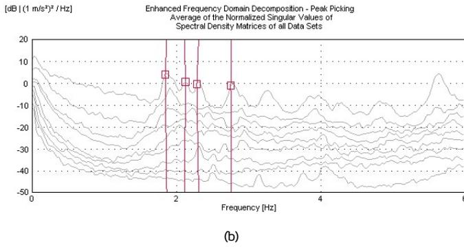
Figure 4. (a) ANSVSDM and (b) SVSDM of the data sets obtained from the EFDD method
