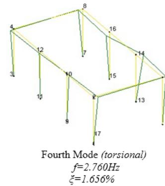
Figure 5. The experimental modal characteristics of the building
