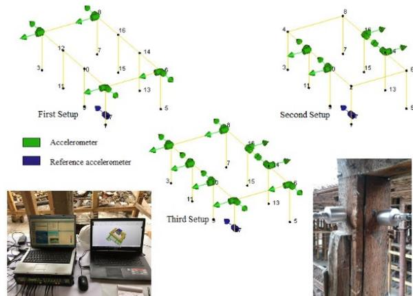
Figure 3. Accelerometer layouts in PULSE software and view of the data acquisition system and accelerometers
