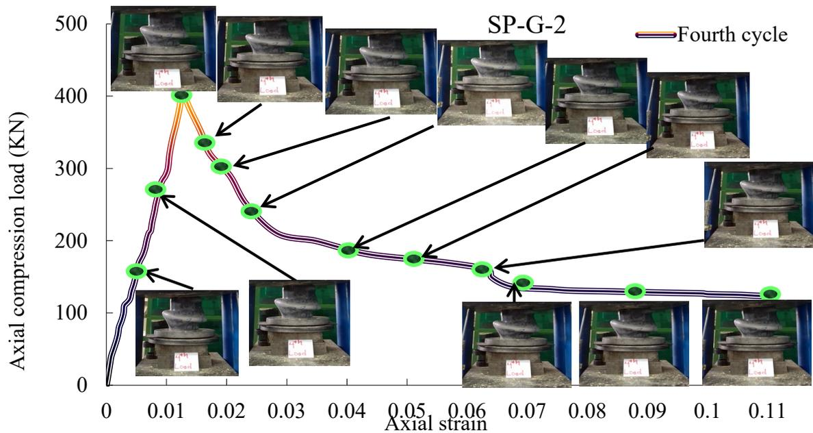
Figure 5. Load –strain relationship for UPVC-confined concrete after fourth cycle of loading
