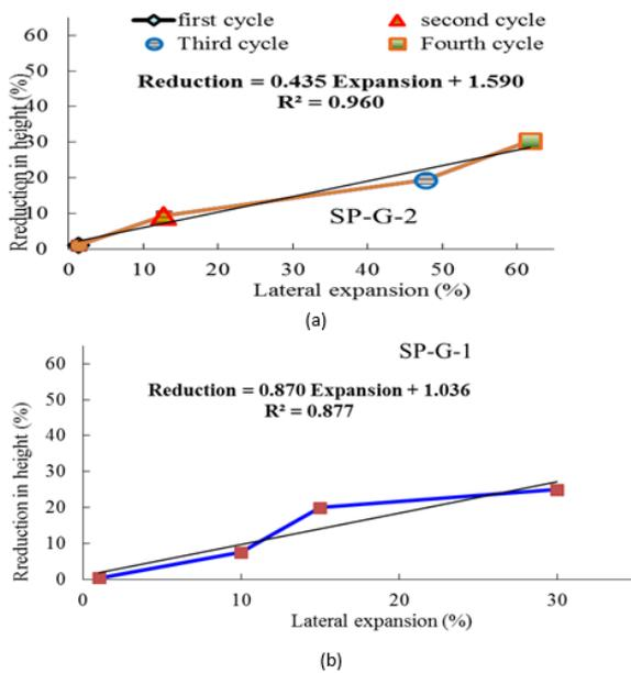
Figure 6. a) Overall reduction in height of specimens versus lateral expansion after each cycle of loading, group two b) Overall reduction in height of specimens versus lateral expansion after each cycle of loading, group one
