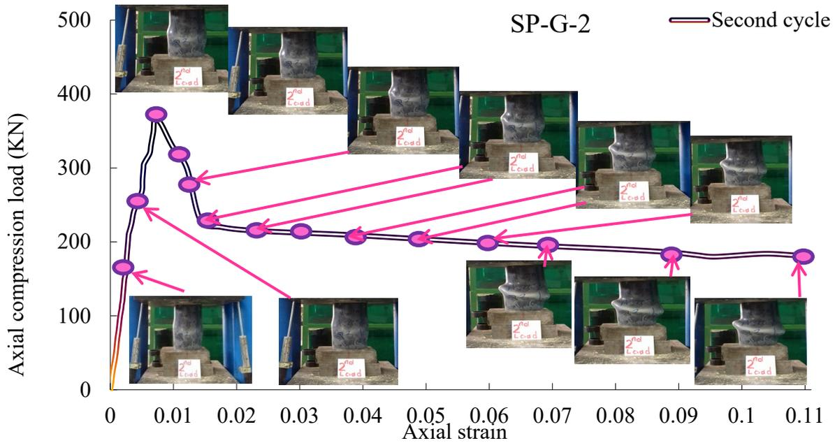
Figure 3. Load –strain relationship for UPVC-confined concrete after second cycle of loading
