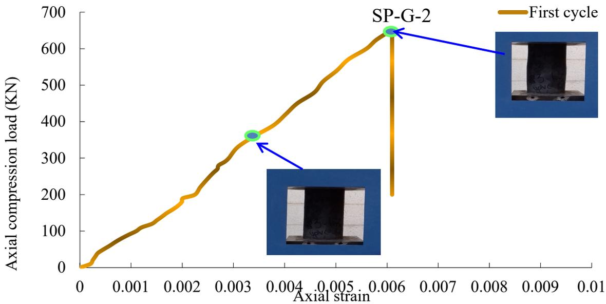
Figure 2. Load –strain relationship for UPVC-confined concrete after first cycle of loading
