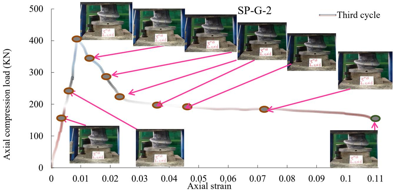
Figure 4. Load –strain relationship for UPVC-confined concrete after third cycle of loading
