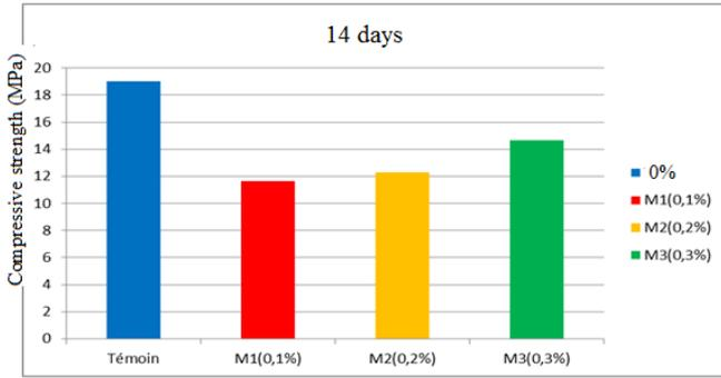
Figure 4. influence of substitution rate on compressive strength at 14 days
