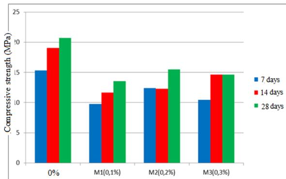
Figure 6. influence of age on the evolution of compressive strength as a function of the substitution rate
