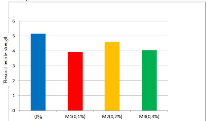
Figure 9. influence of the substitution rate on the flexural tensile strength at 28 days
