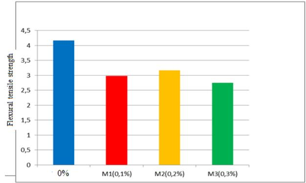
Figure 7. influence of the substitution rate on the flexural tensile strength at 7 days
