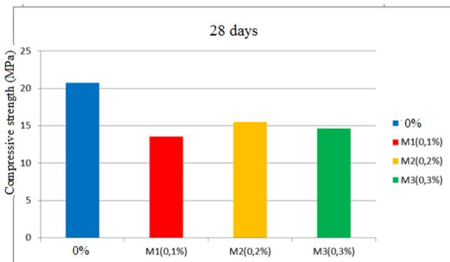
Figure 5. influence of substitution rate on compressive strength at 28 days
