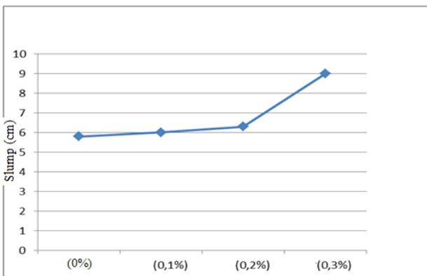
Figure 2. Variation of workability as a function of substitution rate
