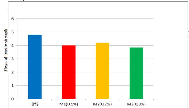
Figure 8. influence of the substitution rate on the flexural tensile strength at 14 days
