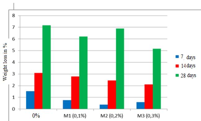
Figure 11. Weight loss depending on the period of immersion in 1% of (H<sub>2</sub>SO<sub>4</sub>) after 28 days in water
