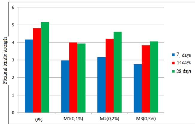
Figure 10. influence of age on the evolution of flexural tensile strength as a function of the substitution rate
