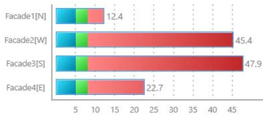
Figure 6. Peak solar heat received by building in Module-2
