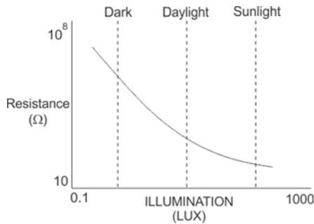
Figure 4. LDR with different sunlight intensity.
