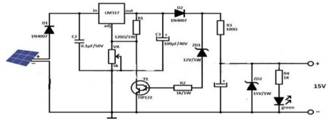
Figure 2. Solar mobile charger circuit.
