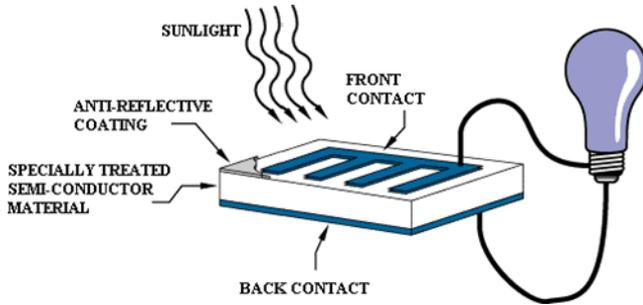
Figure 1. Schematic diagram exhibits the photo voltaic effect.
