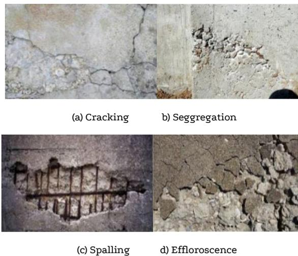
Figure 1. Concrete cracking type
