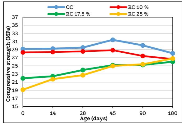
Figure 13. Compressive strength of the mixtures in seawater.
