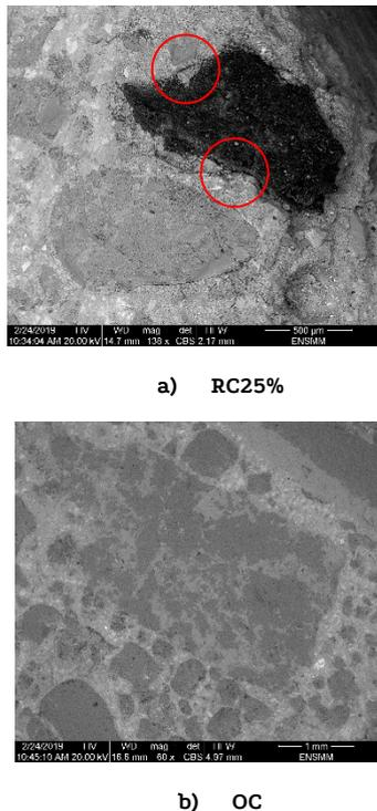
Figure 5. SEM observation of the internal microstructure of the concretes OC and RC25%.
