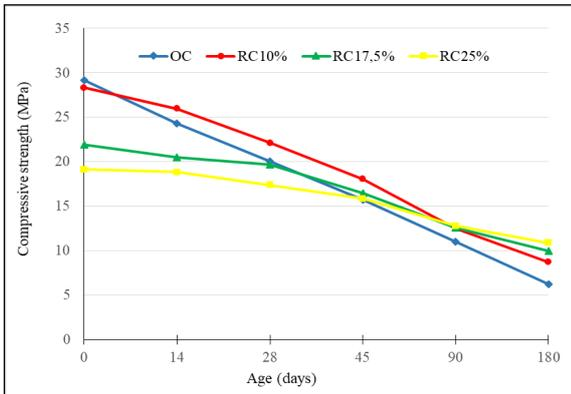
Figure 7. Compressive strength of the mixtures in sulfuric acid.
