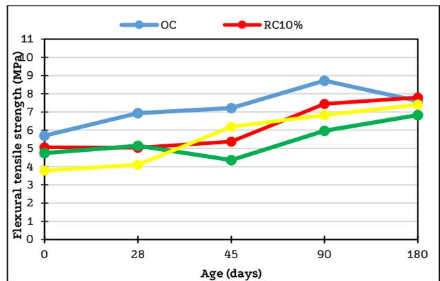
Figure 14. Flexural tensile strength of the mixtures immersed in seawater as a function of curing time.
