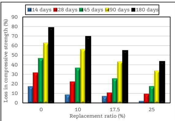
Figure 8. Compressive strength loss of acid attacked specimens.
