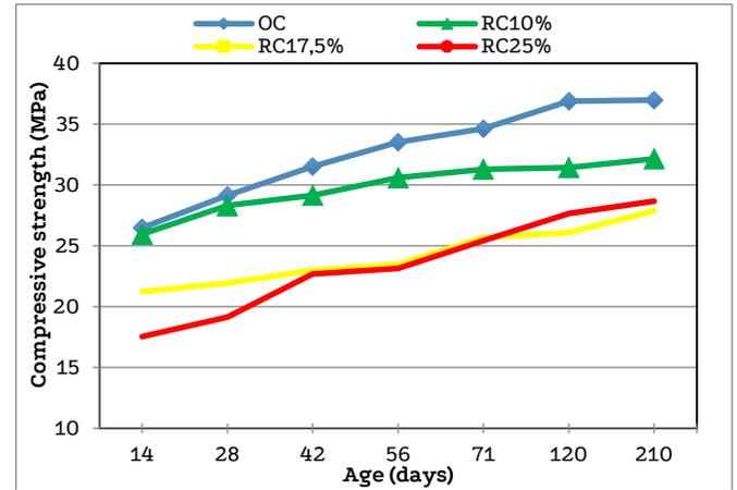
Figure 3. Compressive strength of the mixtures as a function of curing time.
