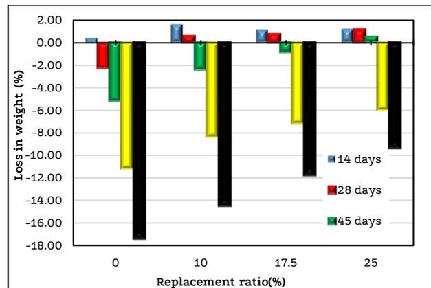
Figure 6. Weight loss of specimens after different age of immersion in sulfuric acid
