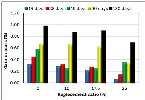
Figure 12. Gain in mass of specimens after different ages of immersion in seawater.
