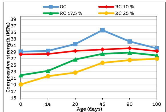
Figure 10. Compressive strength of the mixtures in sodium sulfate.
