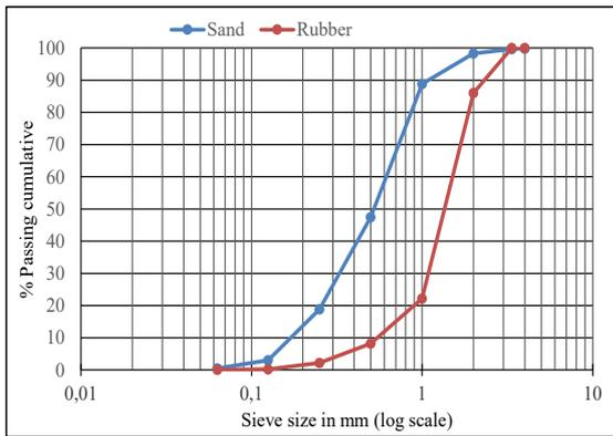
Figure 2. Sieve analysis for sand and rubber used.
