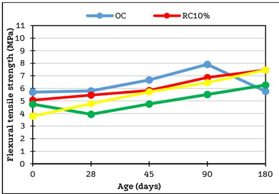
Figure 11. Flexural tensile strength of the mixtures immersed in sodium sulfate as a function of curing time.
