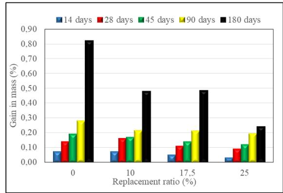
Figure 9. Gain in mass of specimens after different ages of immersion in sodium sulfate.
