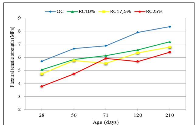
Figure 4. Flexural tensile strength of the mixtures as a function of curing time.
