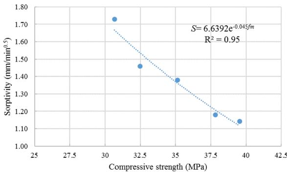
Figure 5. The relationship between the compressive strength of the samples and the sorptivity values
