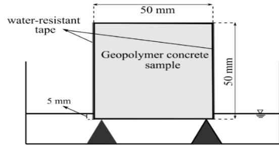
Figure 1. Schematic of the sorptivity test procedure applied to samples
