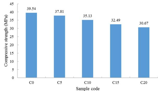
Figure 2. Compressive strength values of the samples
