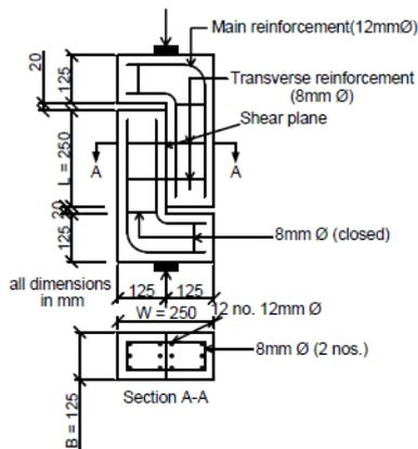
Figure 1. Details of test model
