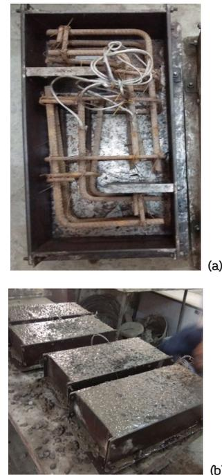
Figure 2. Shear-friction specimen(s) (a) before casting (b) during casting
