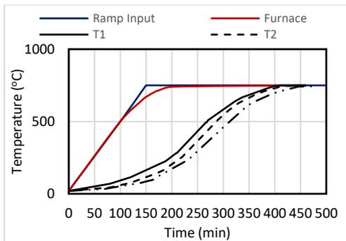
Figure 4. Temperature-Time curve of a specimen exposed to 750°C
