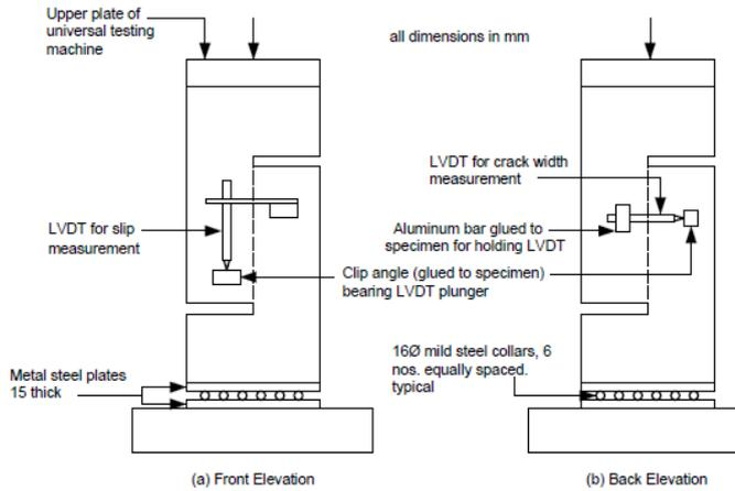
Figure 3. Experimental setup for the determination of shear friction in concrete
