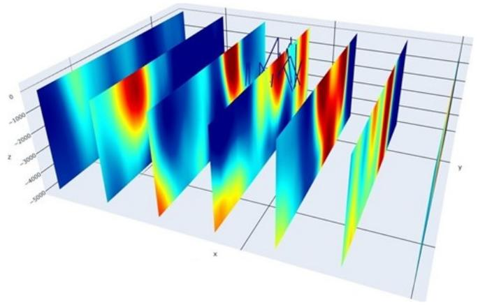
Figure 1. The 2-D visualization of different Vs (m/s) model slices on planar x, y, z coordinates as the latitude, longitude (°), and depth (m) axes for a targeted geothermal area down to ~5.0 km depths. Colors vary from red to blue by indicating low and high velocities [9]
