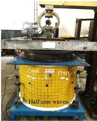
Figure 5. After-test configuration of shell specimen.
