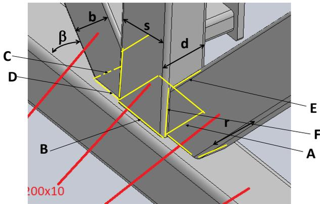
Figure 5. Various welds in 5-member node
