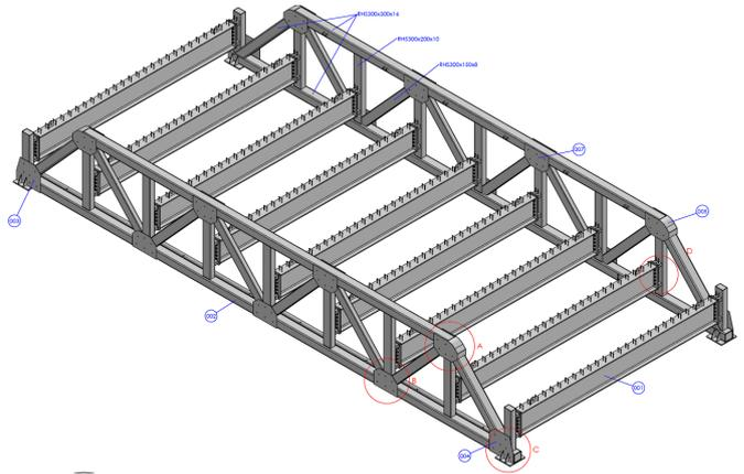
Figure 2. Fabrication model of new truss bridge
