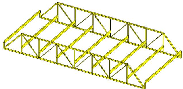
Figure 4. Beam element model of truss bridge
