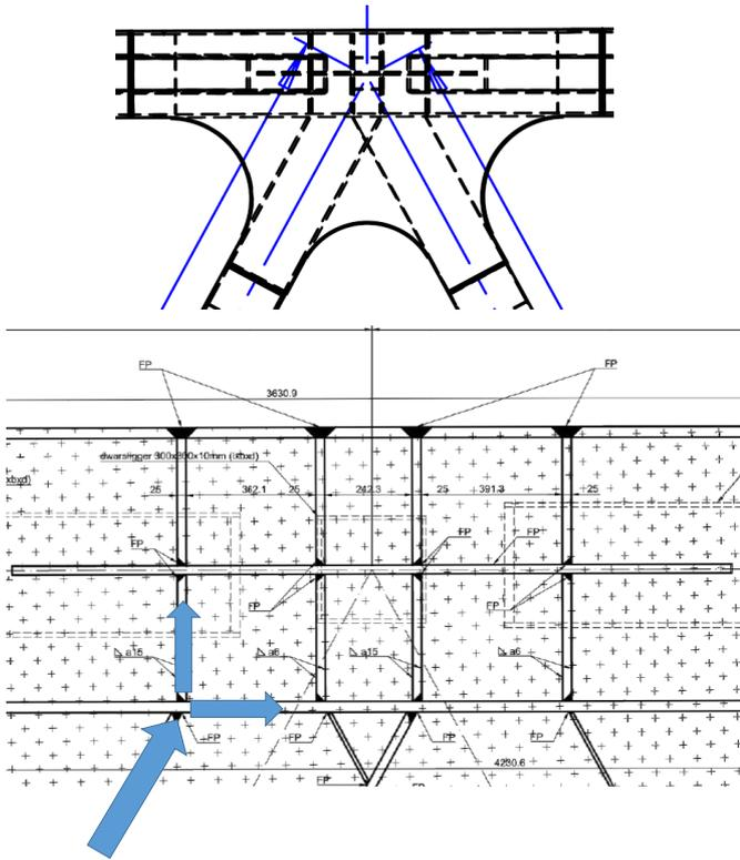
Figure 1. Force transfer in node
