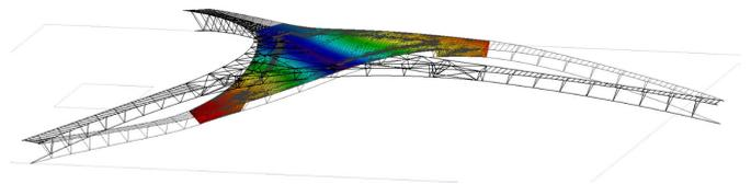
Figure 4. Tripod vibration *modes*
