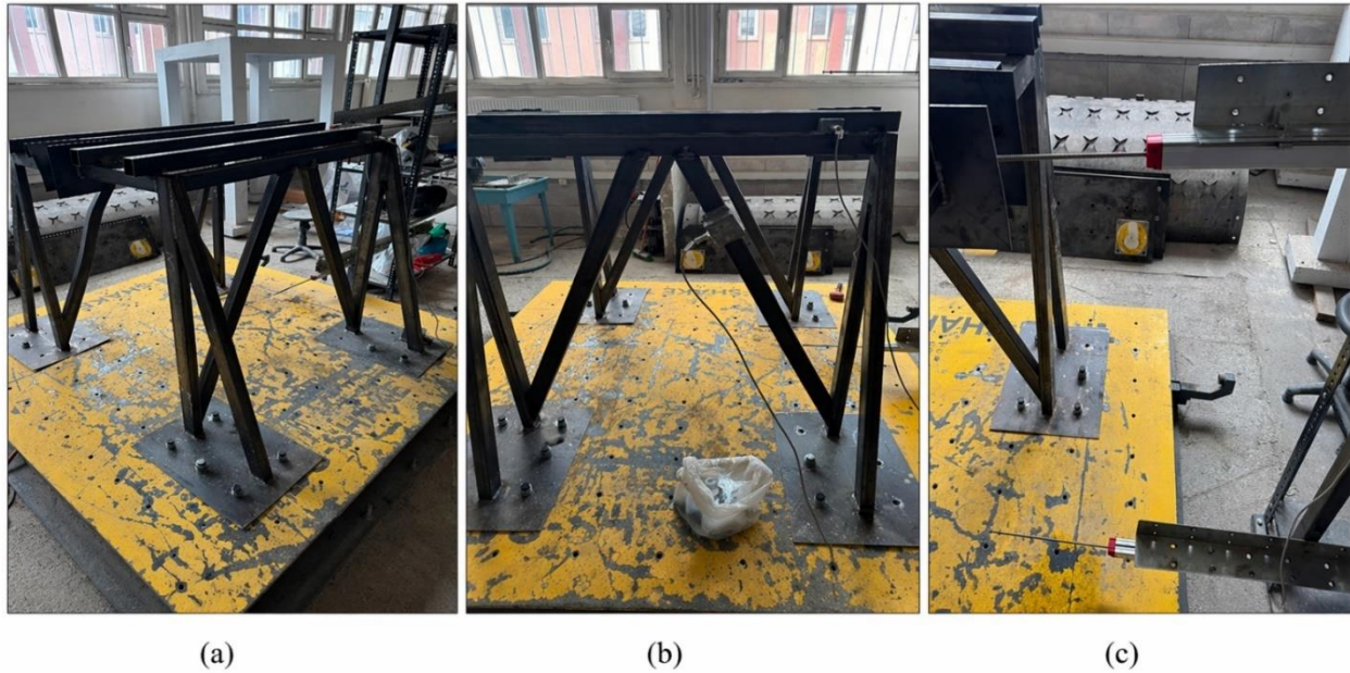
Figure 3. Experimental setup and sensor locations: (a) experimental setup, (b) placement of accelerometers, and (c) placement of the LVDT sensor
