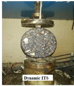
Figure 4. DITS test setup in the PRLS chamber
