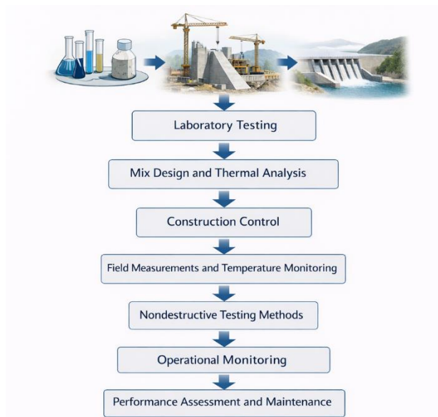
Figure 3. Life-Cycle assessment and monitoring of dam concrete properties
