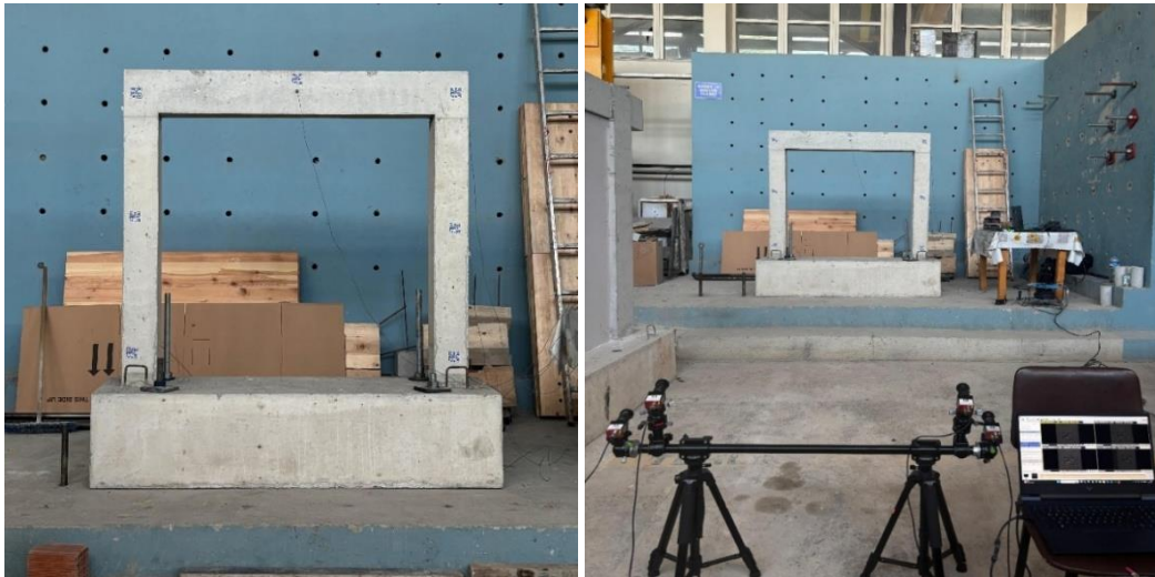
Figure 4. ROI selection and video camera–based measurement setup for the single-story RC frame
