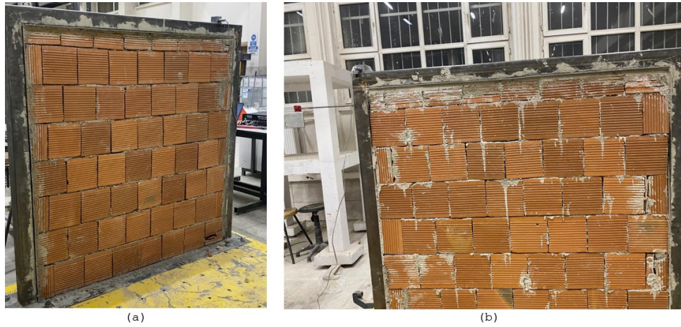
Figure 2. Steel frames with infill walls; a) traditional mortar (TM), b) geopolymer mortar (GM)
