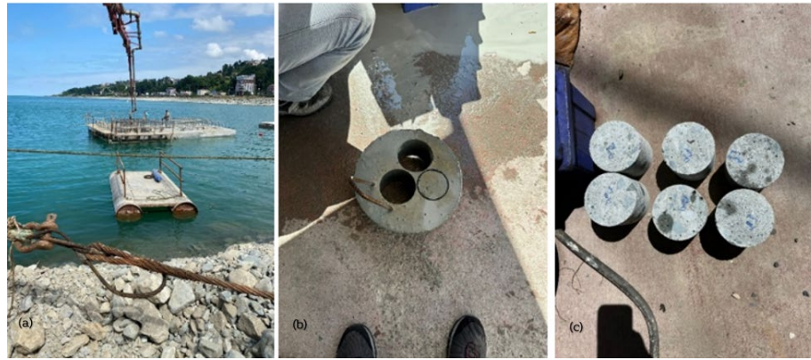
Figure 2. (a) Tremie placement method, (b) core extraction, (c) core samples
