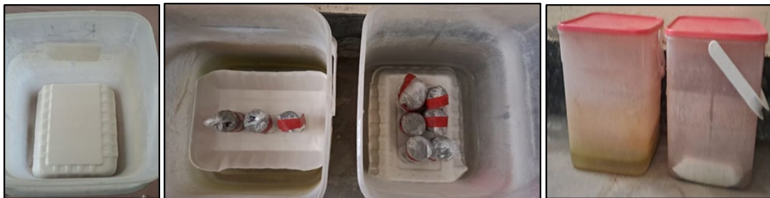
Figure 5. Curing process of UCS sample
