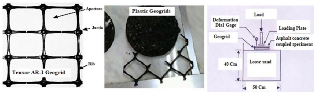
Figure 3. Preparation and testing of geogrid reinforced asphalt concrete samples
