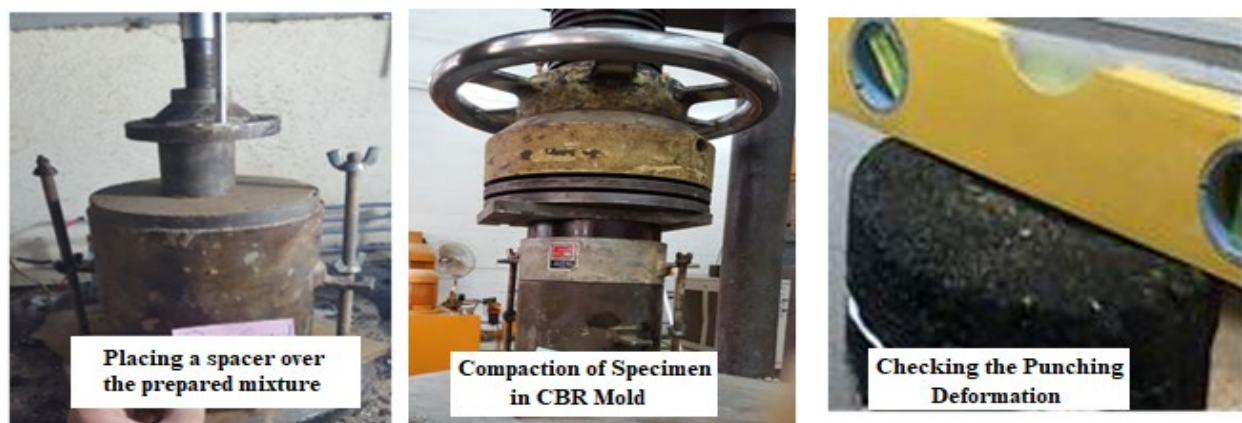
Figure 2. Preparation and compaction of asphalt concrete specimens with the aid of CBR molds and spacers
