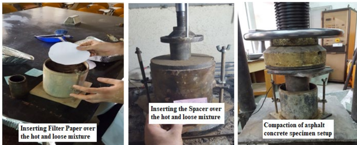
Figure 2. Preparation and compaction of asphalt concrete cylindrical specimens with the aid of CBR molds and spacers
