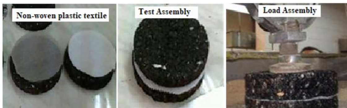
Figure 3. Preparation of geotextile reinforced asphalt concrete samples
