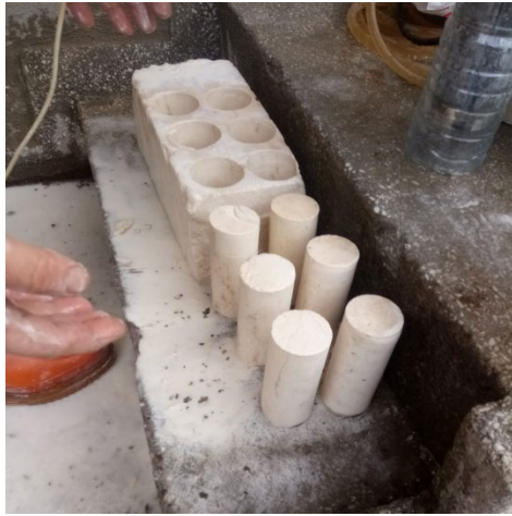
Figure 10. Samples obtained from the minaret body wall stone
