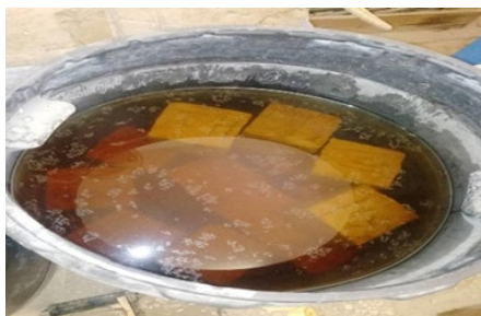
Figure 4. Concrete Samples inside Acidic tank
