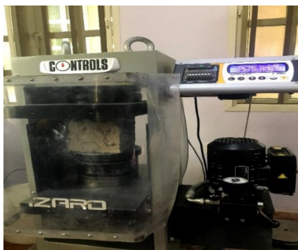
Plate 3. Compressive Strength Test of Concrete Cubes
