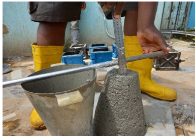
Plate 1. Determination of Concrete Slump
