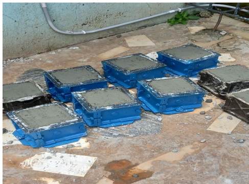
Plate 2. Concrete cube samples in moulds
