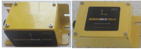
Figure 1. Accelerometers used in the experimental study
