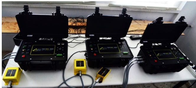
Figure 2. Dynamic data acquisition device and acceleration recording system
