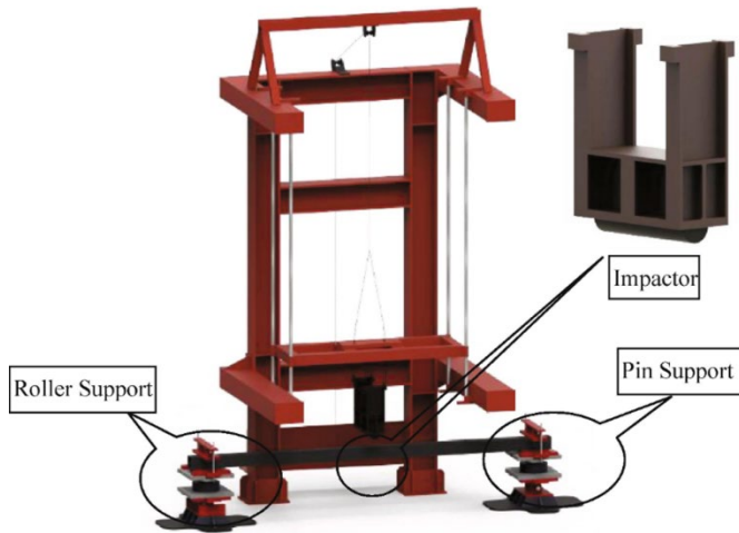
Figure 1. A three-dimensional view illustrating the experimental setup [22]
