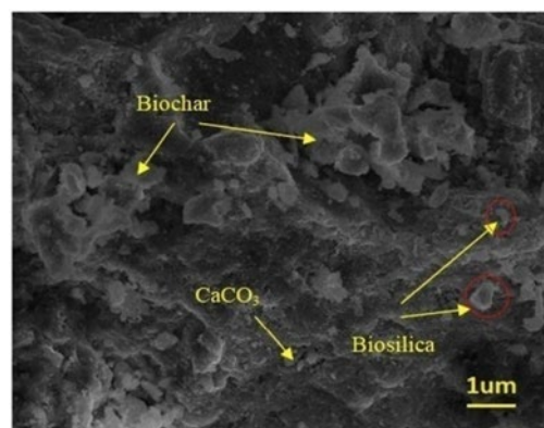
Figure 4. The SEM picture of biocement made by means of exploratory arrangement 10
