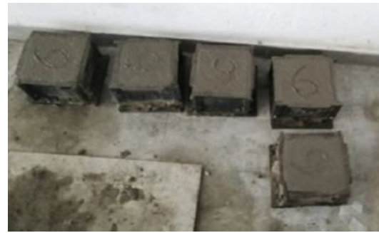
Figure 2. Biocement concrete 3D shapes
