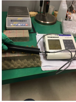
Figure 3. Non-destructive measurements: Wenner resistivity method
