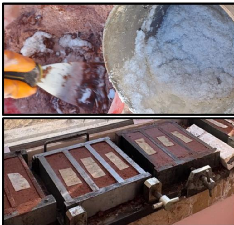
Figure 1. Preparation and molding of the mixture.
