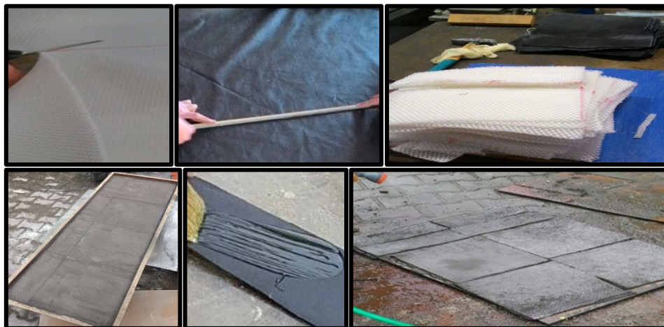
Figure 3. Step-by-step manufacturing process of the 3D textile-reinforced cementitious composite, showing cutting of textile, placement in mold, cement application, and membrane attachment.
