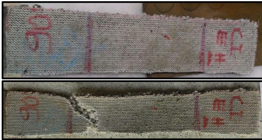
Figure 5. Appearance of 3D textile-reinforced cement composite samples after tensile testing.
