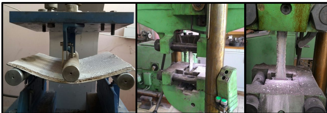
Figure 4. Conducting bending, tensile, and elongation tests on 3D textile-reinforced cement composite samples.
