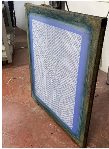
Figure 2. Photograph of the screen-printing process used to fabricate the FSS on a textile substrate
