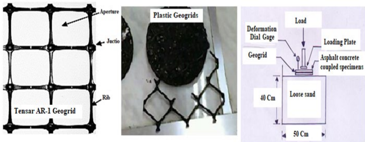
Figure 3. Preparation and testing of geogrid reinforced asphalt concrete samples
