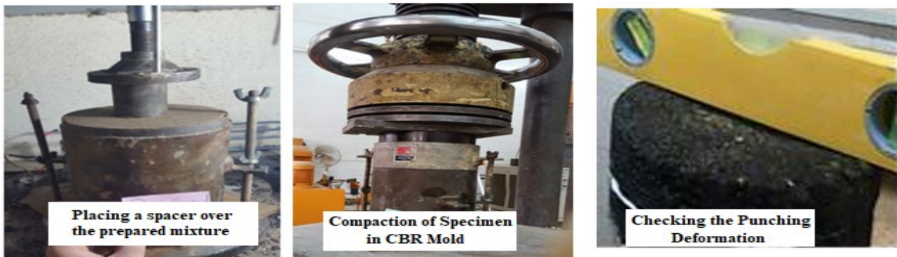
Figure 2. Preparation and compaction of asphalt concrete specimens with the aid of CBR molds and spacers
