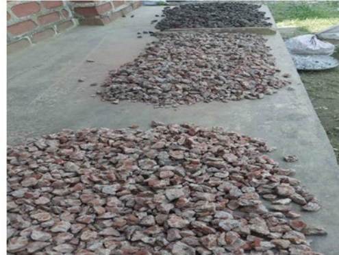
Figure 1. Recycled concrete aggregate
