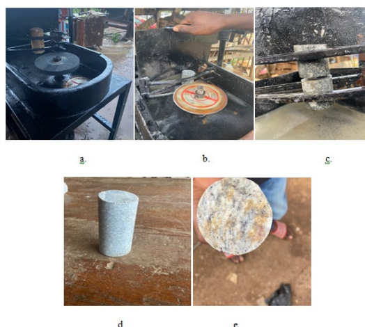
Figure 6. Pictures of the machine set up, polished sample and cutting samples
